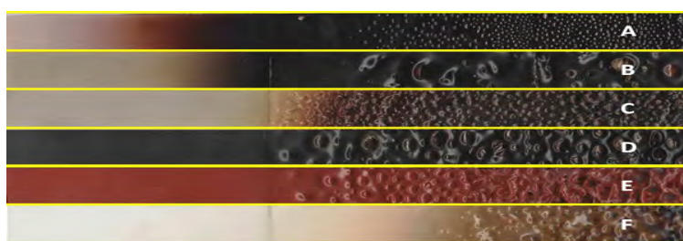
Figure 1: Metrastat sample appearances. (A) Neat PVC; (B) MgAl-LDH; (C) CaAl-LDH; (D) MgCuAl-LDH; (E) MgFeAl-LDH, and (F) MgZnAl-LDH
